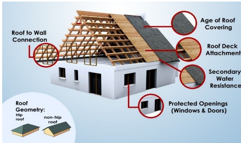
Figure 9: Severe wind mitigation efforts applied to residential home (Tallahassee Real Estate Inspections LLC)
